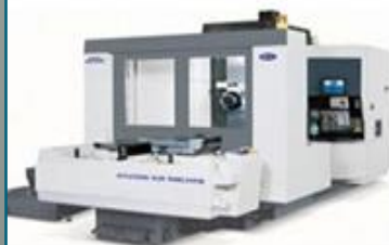
HORIZONTAL CNC MACHINING CENTER (WIA, KH63G) - 950 x 825 x 760
