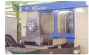
HORIZONTAL MACHINING CENTER (WIA, HC-800) — 1,250 x 950 x 900 — 5축 가공 가능
