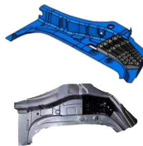
Multi-material A- Pillar (Steel + CFRP + GFRP)
