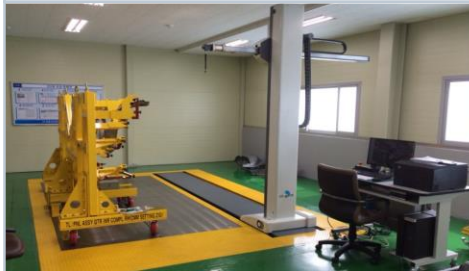
CMM (3-D measuring machine)
