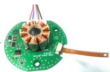
BLDC (Brushless DC Electric motor)
