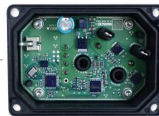
ACU (Actuator Control Unit)
